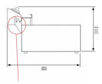
TILT UP ELEMENT HEAD WITH SAFETY LOCK DEVICE
